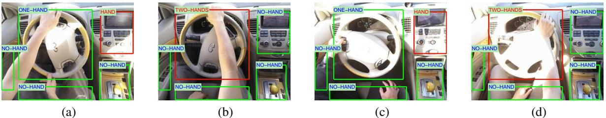
Figure 5: Incorrect classification using the proposed system. (a) Although the wheel model outputs a prediction of two hands in the wheel region, so does the infotainment due to an illumination artifact. In this case, the integration produces incorrect results since the model learns to give high confidence to the infotainment score. (b) The lap region produces incorrect classifications due to poor separation in the feature space. (c) and (d): Illumination produces false positives.
