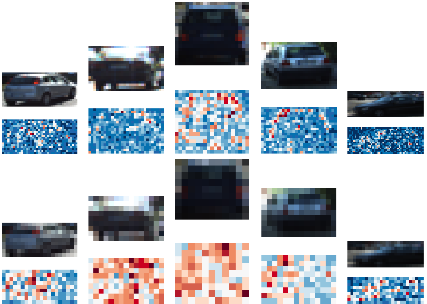
Fig. 15: Learning components at multiple resolutions (visualized here for widths 64 and 32 pixels in the top and bottom row, respectively) with the hybrid multiresolution approach results in significant performance improvement. Warmer colors correspond to feature locations with more attention given by the classifier.
