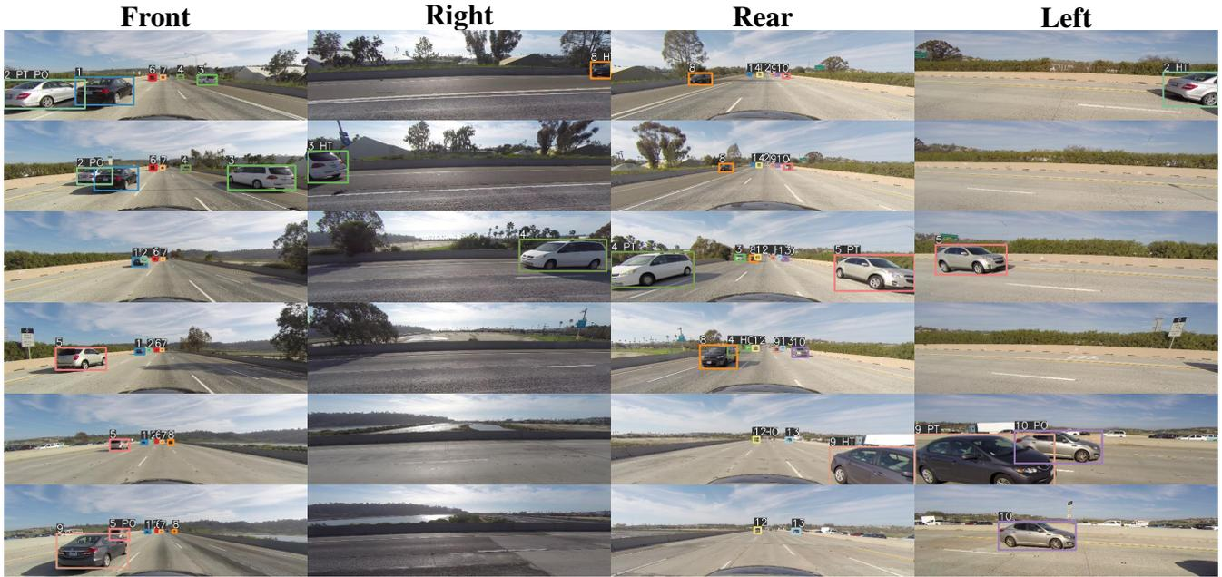
Fig. 2. Sample images from one of the sequences in the dataset with overlaid ground truth annotations at six different time instances. The bounding boxes are color coded by *id* and labeled with *PO*, *HO*, *PT*, and *HT* denoting partial occlusion, heavy occlusion, partial truncation and heavy truncation, respectively.
